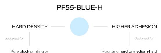
Pure **block** printing or combination of **both half-tone and block** printing when used on the same plate. Mounting hard to medium-hard photopolymer and rubber clichés on to small to medium size diameter cylinders.
